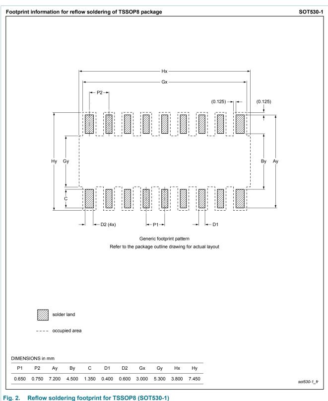
plastic, thin shrink small outline package; 8 terminals; 0.65 mm pitch; 3 mm x 4.4 mm x 1.1 mm body
